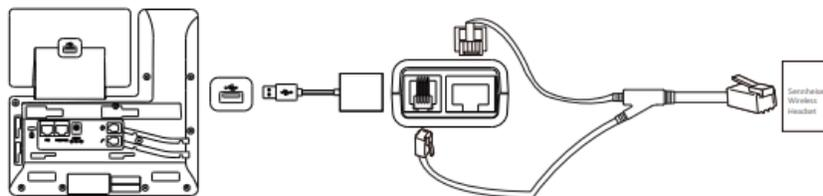
The following figure shows the connection between the IP phone and the Plantronics wireless headset.
