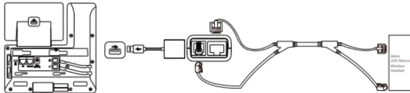
The following figure shows the connection between the IP phone and the Sennheiser wireless headset.
